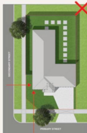
Diagram 5 – Flat façade does not address the primary and secondary frontages
