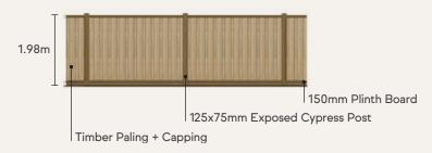
Note: all other internal boundary fencing to be typical maximum 1.98 metre timber fence with capping and exposed post.
